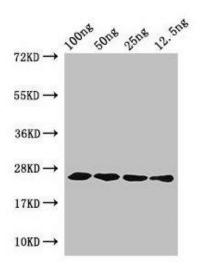
Western Blot. Positive WB detected in Recombinant protein. All lanes: hfb1 antibody at  $4\mu$ g/ml. Secondary. Goat polyclonal to rabbit IgG at 1/50000 dilution. predicted band size: 25 kDa. observed band size: 25 kDa.
